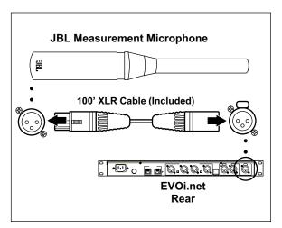
Figure 5 - Measurement Microphone Hook Up
